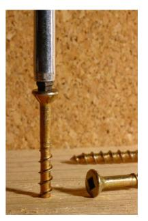
When boards of equal thickness have to be joined, a screw length should be selected that is approximately 30 millimetres less than the combined thickness of the parts. The general rule that should be adhered to is that for components that differ in size, approximately two-thirds of the screw length should penetrate the thicker component.
